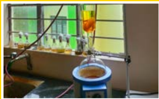
Figure 2: Extraction of Curcumin using the Soxhlet apparatus
