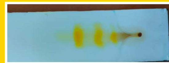
Figure 7: Separation of the three curcuminoids by TLC (Thin layer Chromatography); namely Curcumin, Demethoxycurcumin(DMC) and Bidemethoxycurcumin (BDMC)
